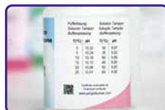
Value table depending on temperature and QR Code with link to our website
